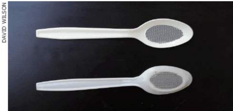
Figure SOP 2.1. “Net spoon” for removing bee specimens from traps/bowls (Wilson 2009).
